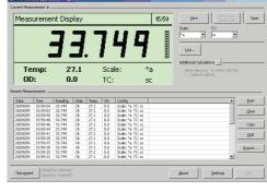
The instrument can be checked and calibrated using a quartz control plate by accessing the span facility in the setup menu. If a sample is too dark, the instrument will display an error message.
