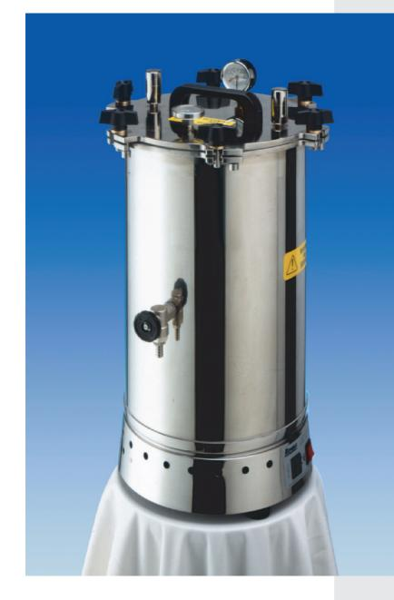
**Compact and Fully Portable Electronic Temperature Control** Simple and Safe Use **Domestic Electricity Supply** No Plumbing Needed **Minimal Maintenance Required** Electrically Safe To BS3456 Lid Locking Safety to H&SE PM73 Produced under ISO 9001 Suitable for Culture Media 121°C Operating Temperature 316 Stainless Steel Construction 22 Litre Capacity 280mm Internal Diameter 21.0Kg Net Weight **CE Marked**
