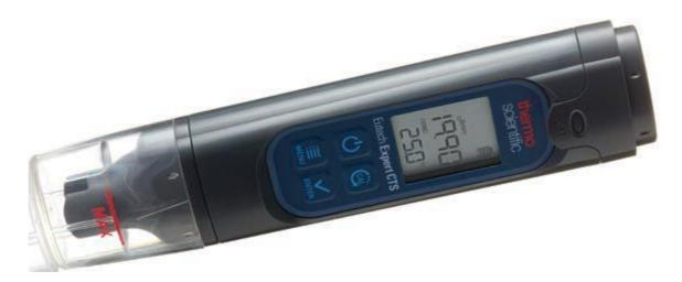
Eutech Expert CTS tester accurately measures conductivity, TDS, and salinity in one single instrument, with ATC, an ideal solution for many applications.
