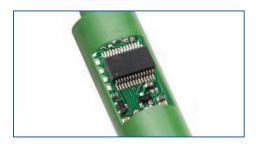
edge measures pH through its unique digital electrodes. Connected via an easy plug-in 3.5mm connector, these smart electrodes enable edge to automatically recognise and store sensor type, ID and calibration information.
