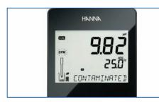
edge warns users if the electrode is not clean or if buffers are contaminated during calibration using the exclusive HANNA CAL-CHECK feature. Advancing this technology even further, edge will also warn you if the pH bulb is cracked or if the junction of the electrode is compromised.
