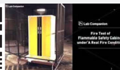
Fire simulation test (90mins)
