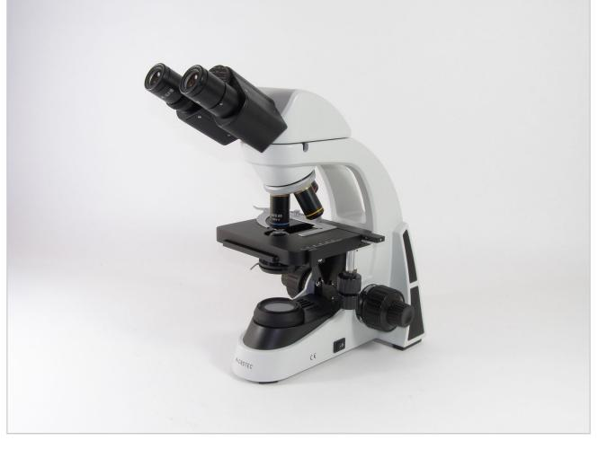
The PM-6 microscope is an economically priced instrument but with a performance for exacting microscopy. The focusing Abbe condenser provides suitable illumination for use with the 100x oil objective. The built in long life LED illumination provides bright even illumination.
