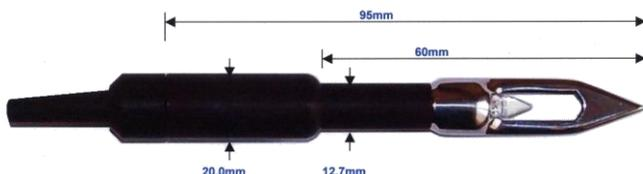
These combination electrodes, employing the use of solid gel, were designed with the water industry very much in mind. Capable of being used with portable instruments, and on-line, they will give optimum performance in cold water. The gel retains salt, and maintains zero potential for a much longer period of time. The mechanical strength of the gel allows the use of a junction with a much higher porosity than previous designs. This benefits the user in the following ways:
