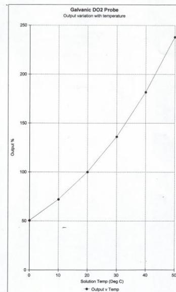
*output approx 45mV at 20°C with 5K Resistor*
