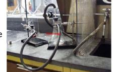
Only use this set-up if your solvent is non-volatile and non-hazardous, such as water. Methylene chloride and similar solvents will be drawn out of the flask and end up in the water being flushed down the drain through the water aspirator.
