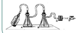
A suction flask is used to collect the contaminated fluids into a suitable decontamination solution. A second flask serves as a fluid overflow collection vessel and an in-line HEPA filter is used to protect the vacuum system from aerosolized microorganisms.
